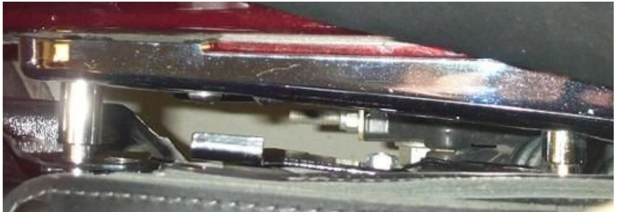
Step D. Push the locking / safety lever on the inside of the bag to the down position.
