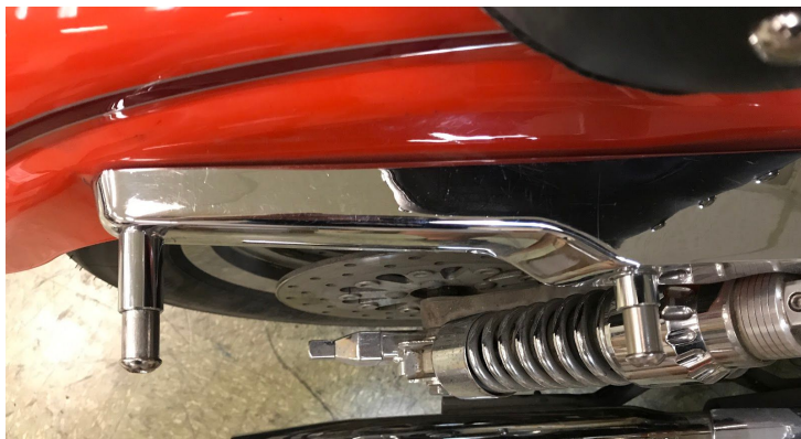
Correct mounting of docking points.
