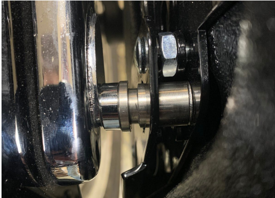
INCORRECT Brackets are not on the docking points and will not clamp on in this position
